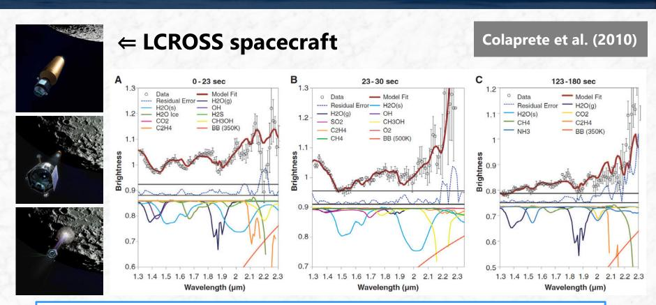
Near Infrared (NIR) spectrometer found the water bands
